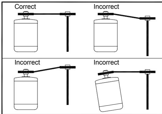
Figure 9 - Pulley Alignment
