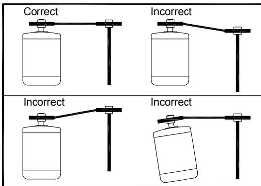
Figure 9 - Pulley Alignment
