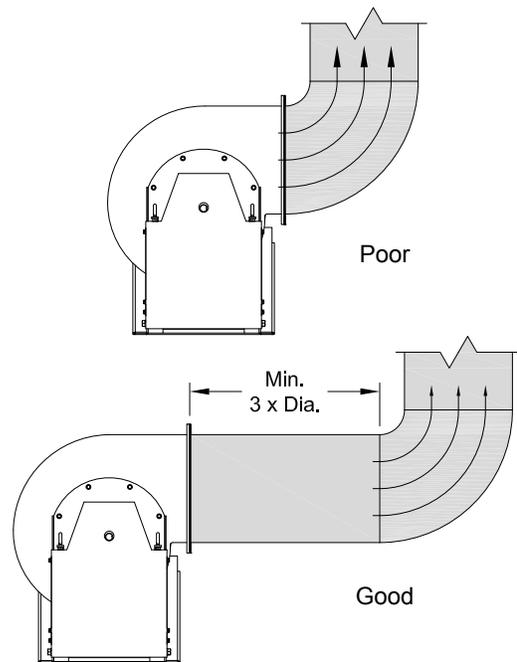
Figure 4 - Outlet Ducting
