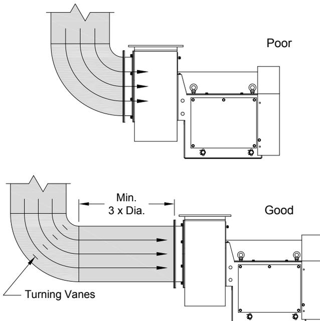
Figure 2 - Inlet Ducting
