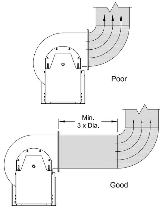
Figure 4 - Outlet Ducting
